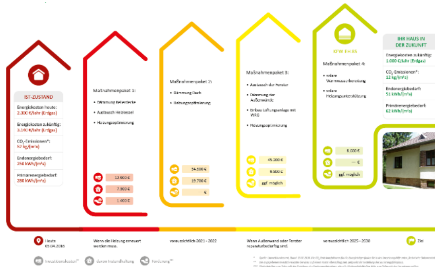
Figure 11: iSFP - renovation roadmap
